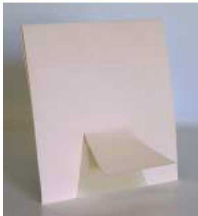
Figure 5a Folded over to provide stiffness and the prop cut out rather than added on
